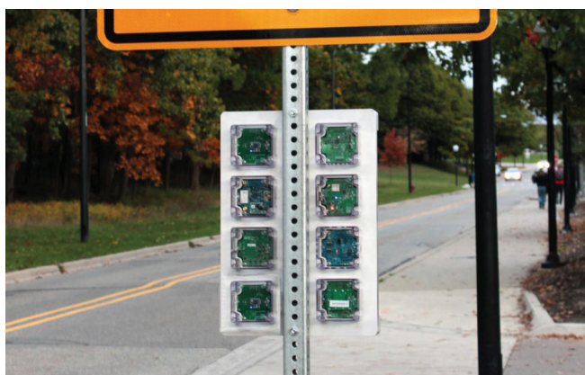
FIGURE 1. The Signpost platform easily mounts to existing street sign posts, harvests energy from an integrated solar panel, and provides pluggable sensor modules with power, communications, processing, storage, time, and location. Signpost is open source, with all hardware and software available on Github.
